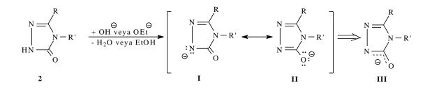
The resonance hybrid of I and II resonance structures is III, showing that the negative charge is delocalized to include electronegative nitrogen and oxygen atoms.
