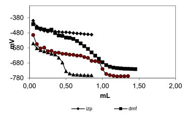
**Figure 1**. Potentiometric titration curves of 0.001 M solutions of compound **3** in 10<sup>-3</sup> M solutions of DMF, acetonitrile, isopropyl alcohol, and tert-butyl alcohol with 0.05 N TBAH
