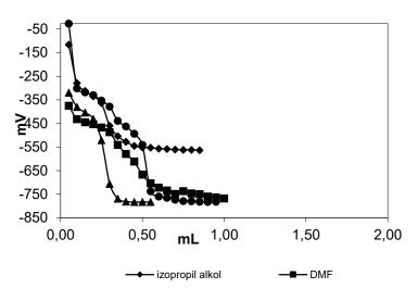
**Figure 5**. Potentiometric titration curves of 0.001 M solutions of compound **7** in 10<sup>-3</sup> M solutions of DMF, acetonitrile, isopropyl alcohol, and tert-butyl alcohol with 0.05 N TBAH
